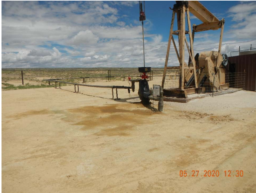
Photo 2. Stained soil at wellhead.
