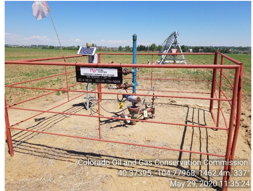
Photo 2: Wellhead; equipment removed
