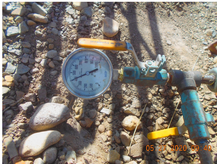
Wellhead gauge at end of test
