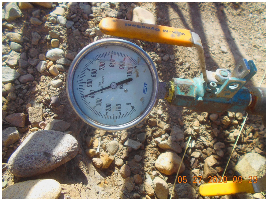
Wellhead gauge at 5 minutes
