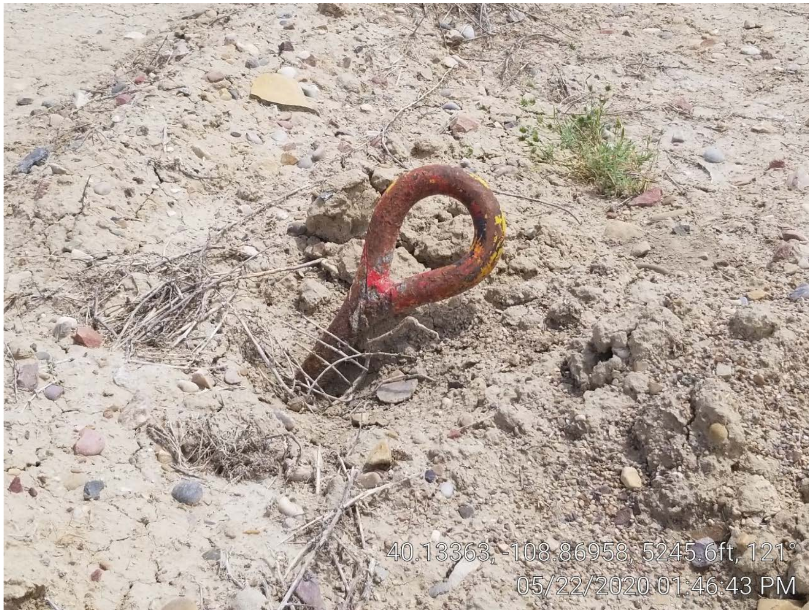
Photo 2. Unmarked deadman in SW corner.
