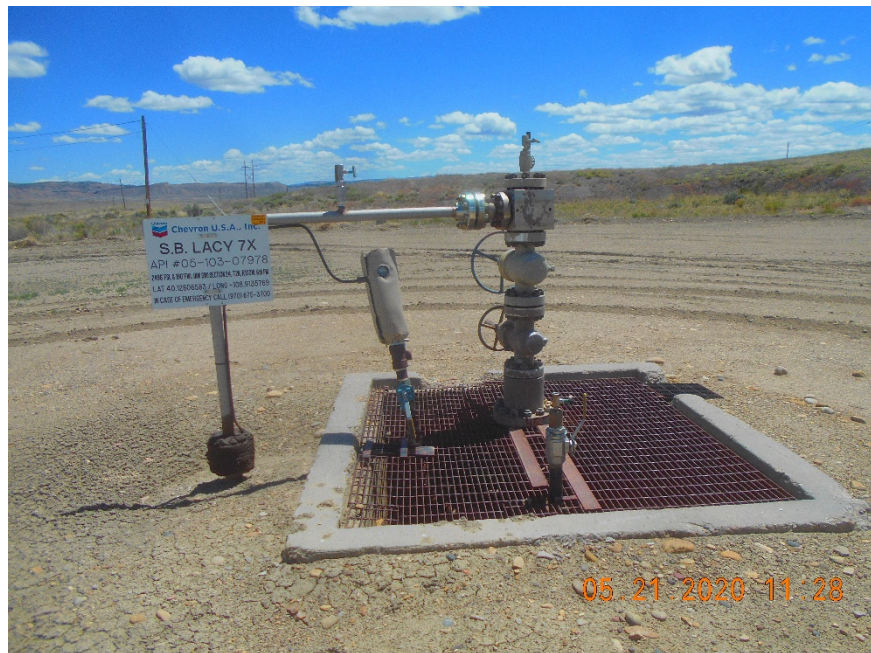
Injection wellhead
