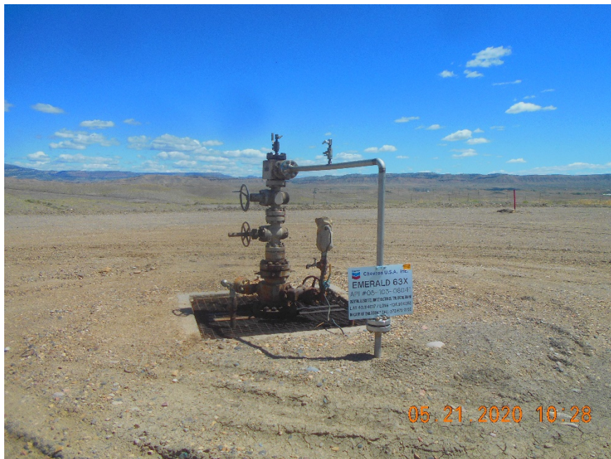
Injection wellhead
