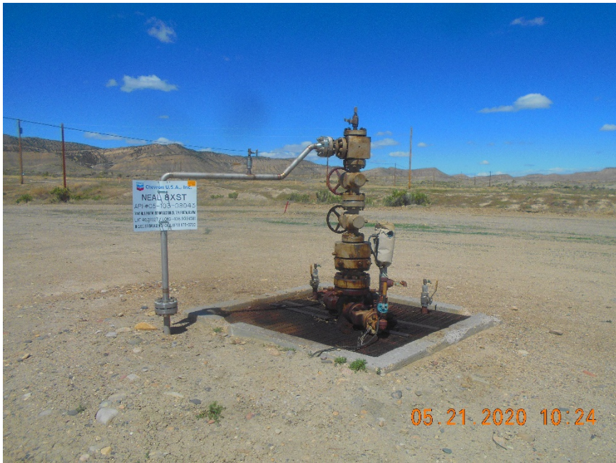
Injection wellhead
