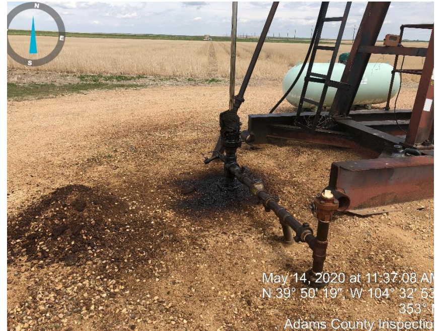
Photo #2 stained soil at well head
