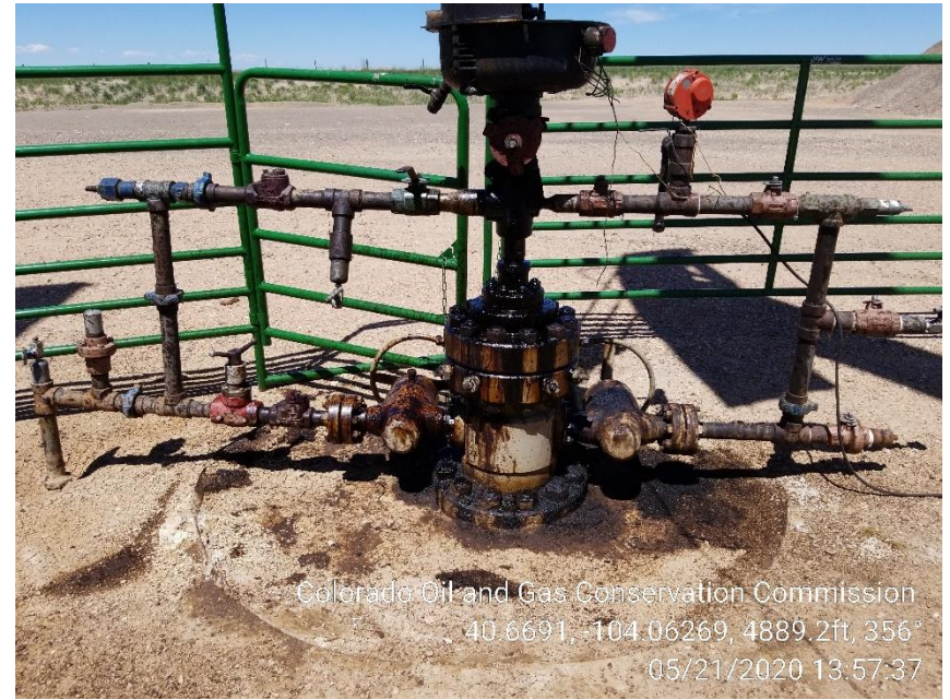
Photo 4 – Stained Soil at 2-14-8-60 Wellhead
