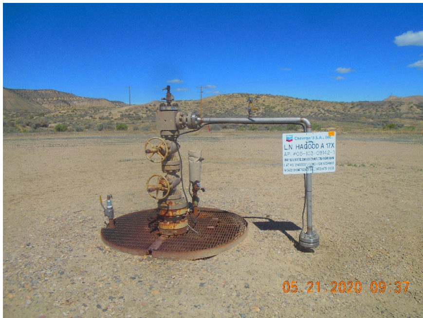
Injection wellhead
