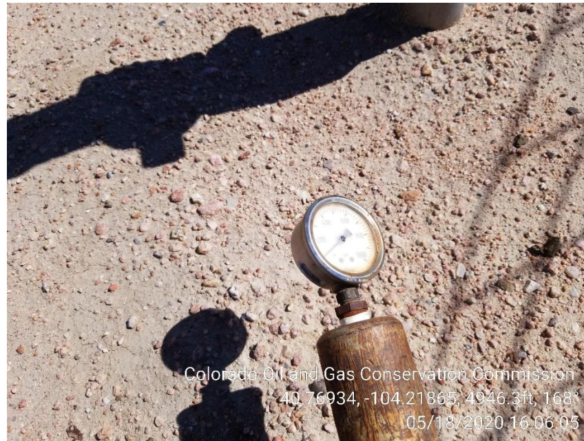
Photo 4 – Casing Gauge
