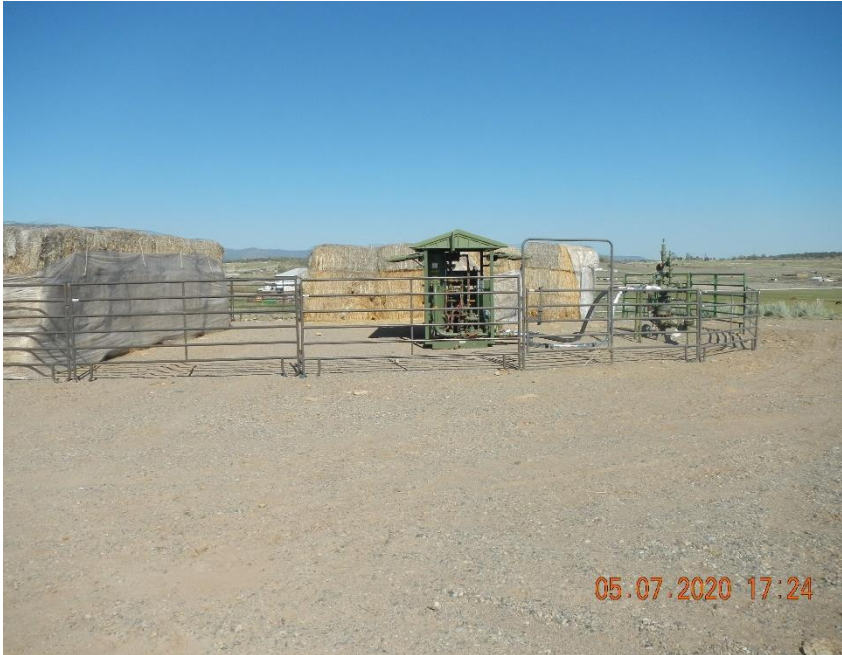
McCaw C #1 well head and skid mounted compressor.
