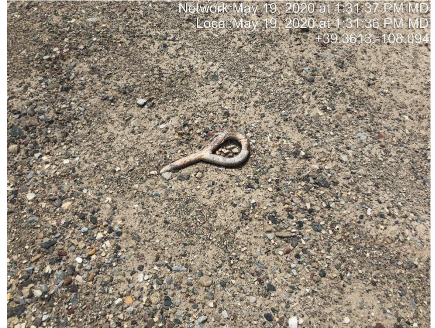
Photo #1222 Multiple unmarked deadman.
