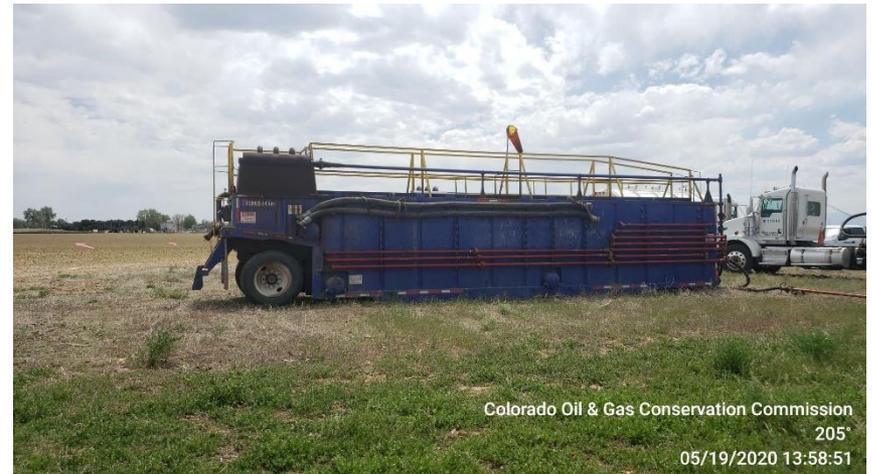
**Photo 3 Nextier Cement pumping unit, Ensign workover Rig mud pump**
