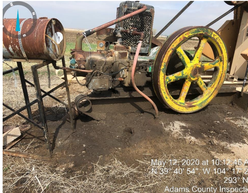
Photo #7 stained soil next to Pump Jack motor
