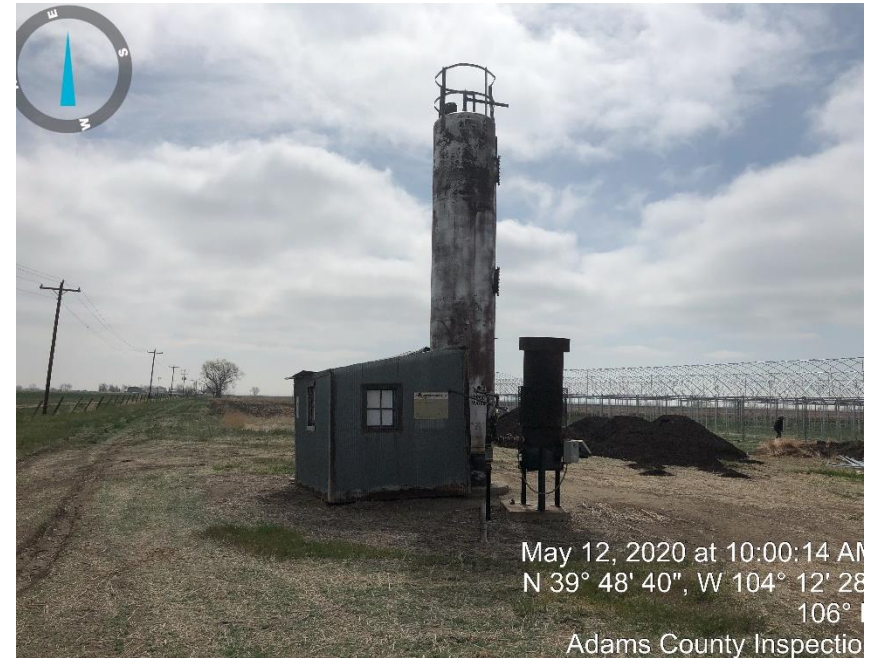
Photo #4 vertical separator & EDC
