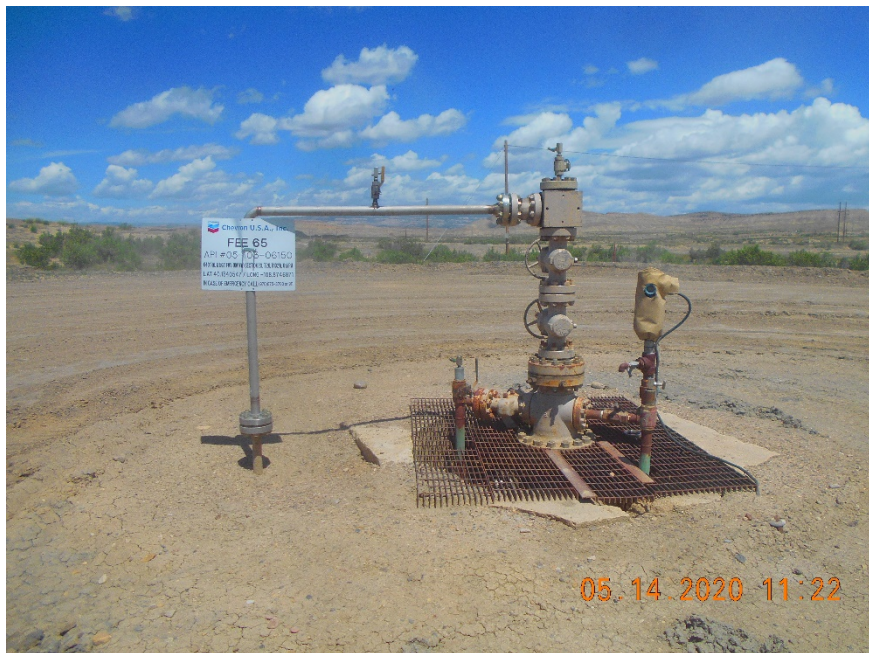
Injection wellhead
