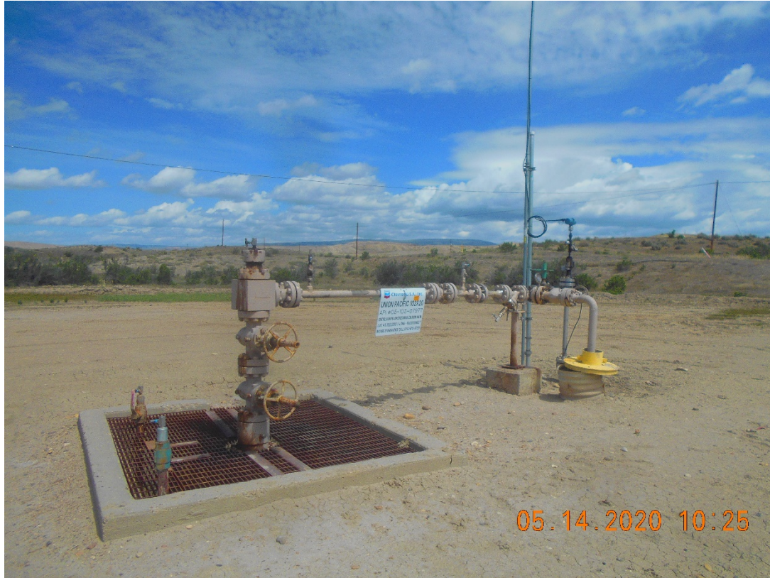
Injection wellhead
