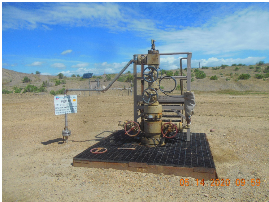
Injection wellhead
