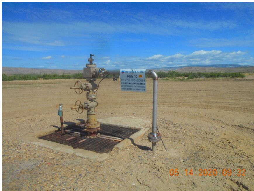
Injection wellhead
