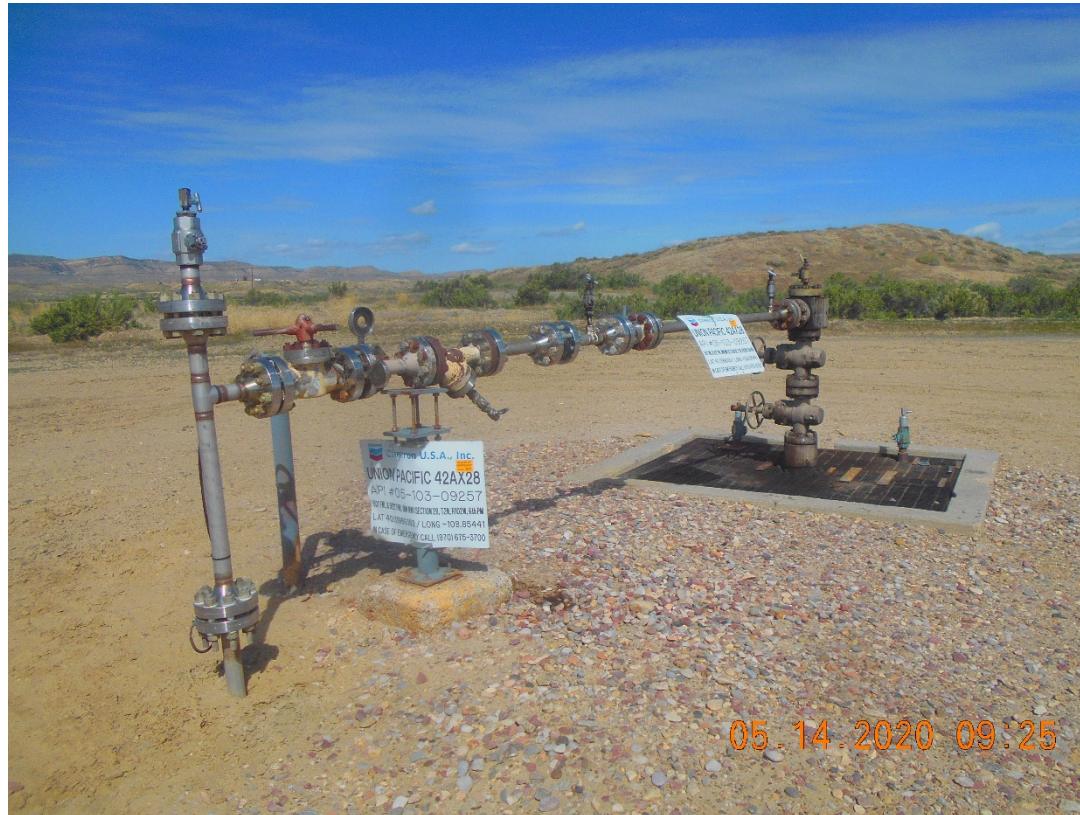
Injection wellhead
