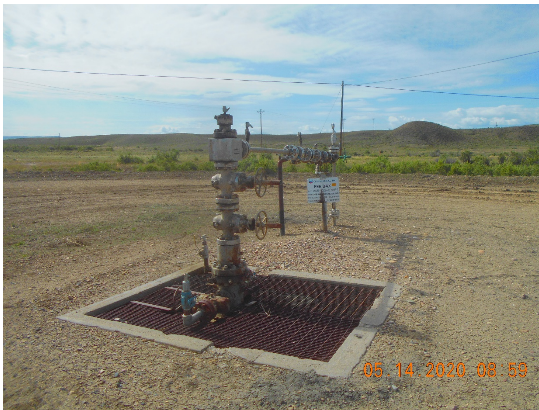
Injection wellhead
