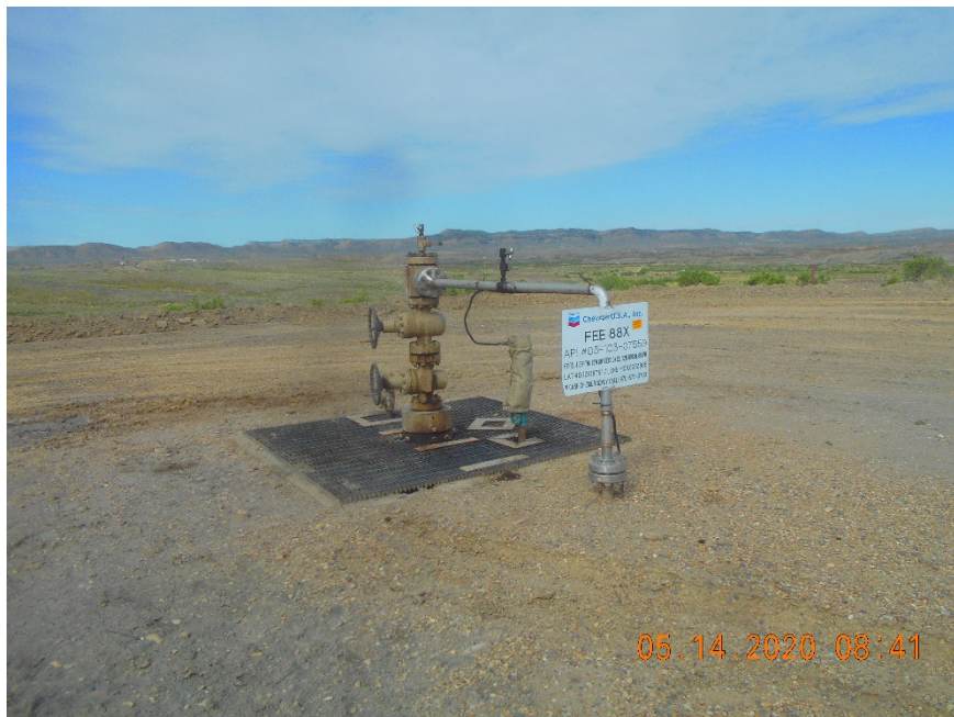
Injection wellhead
