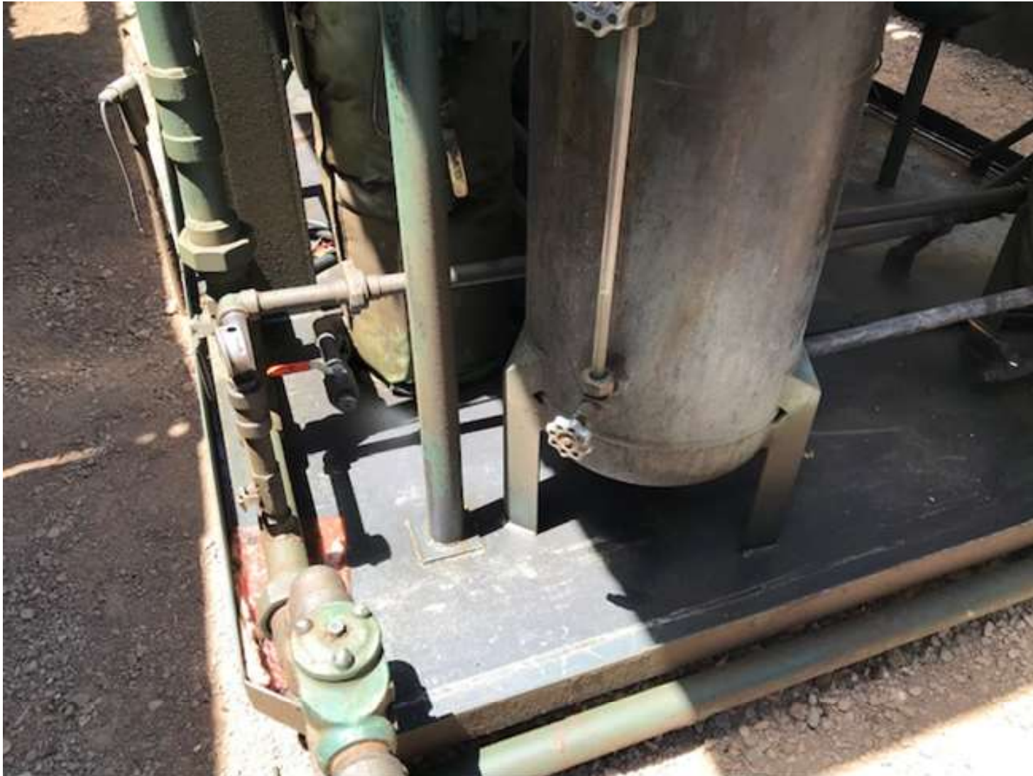
PHOTO 1: THE LEAK ON THE LIQUID RING ENGINE WAS REPAIRED AND THE FLUID ACCUMULATION WAS REMOVED FROM THE COMPRESSOR CONTAINMENT.
