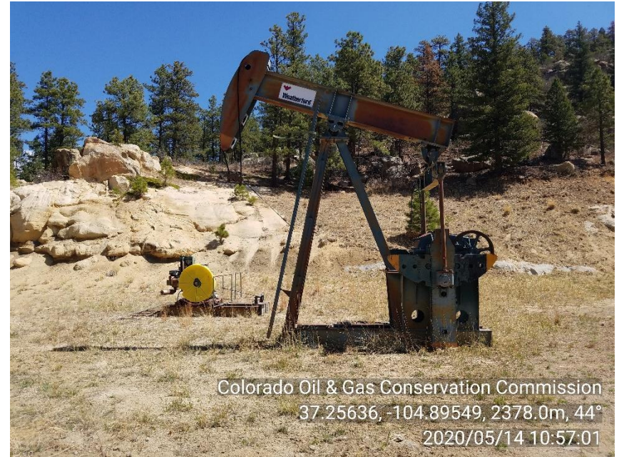
PHOTO 6: UNUSED EQUIPMENT STORED ON LOCATION (PUMPJACK, POWER UNIT FOR PUMPJACK AND LADER). REMOVE UNUSED EQUIPMENT COMPLY WITH RULE 603.f. CA DATE 8-14-20.
