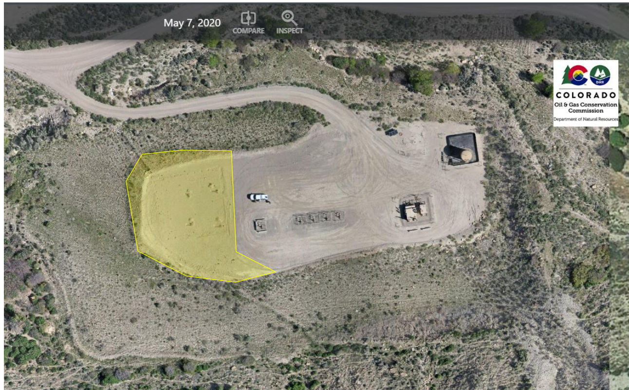
Photo 19: On 5/7/2020, Reclamation Specialist Trujillo utilized a SUA to capture aerial imagery of the Location. Photo shows areas on the west end of the Location where a tank battery existed. Facility has since been removed resulting in areas no longer needed for production subject to 1003 interim reclamation (yellow polygon). Areas are being proposed for use by Operator to store drill cuttings from the NPR 004 Pad, to eventually be utilized for interim reclamation.
