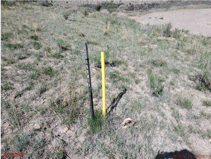
Photo 5: Photo taken from the north end of the Location. Photo shows anchors have been properly marked in accordance with Rule 1003.a
