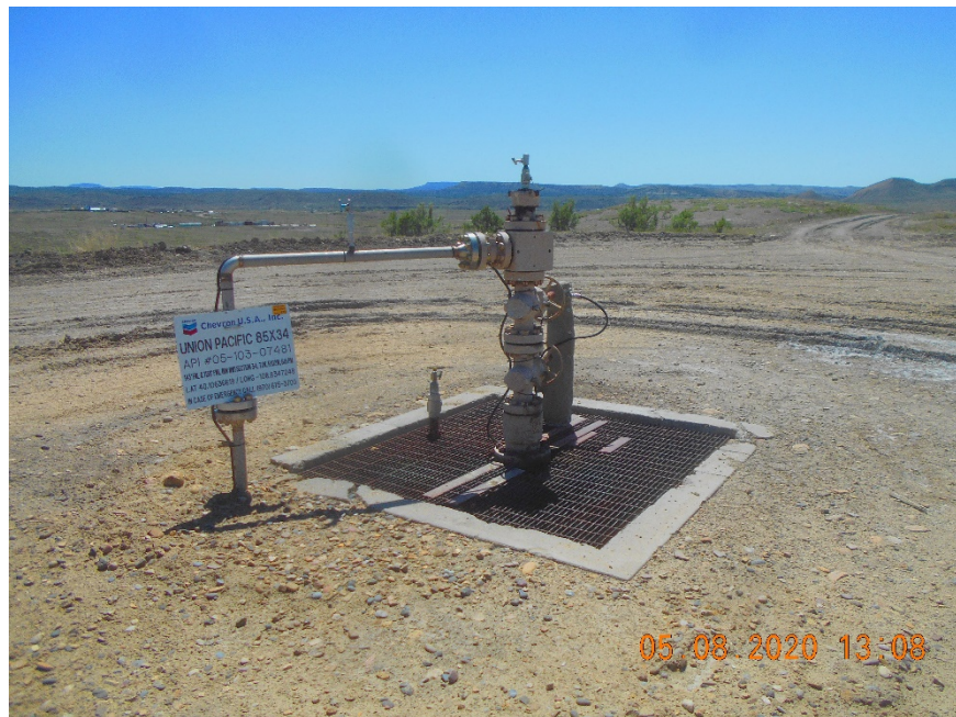
Injection wellhead
