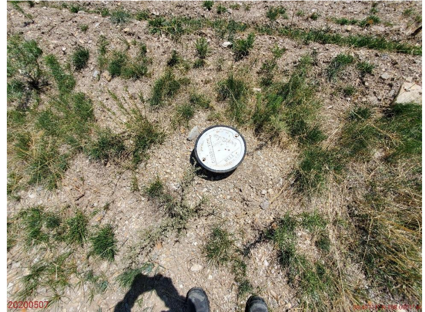
Photo 4: Photo taken from the south end of the Location. Photo shows what appears to be an inclinometer installed to monitor seismic and surface movement conditions of the Location.
