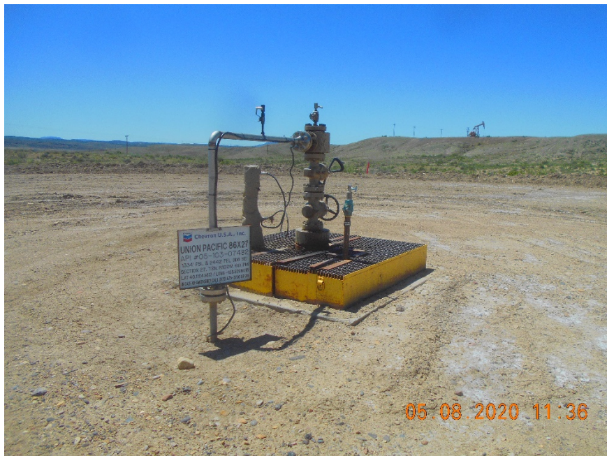
Injection wellhead
