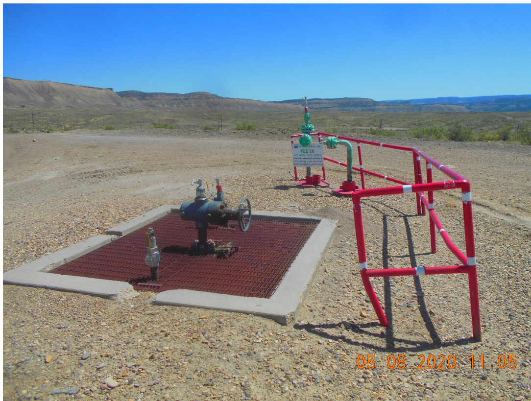
Injection wellhead – Temporarily Abandoned
