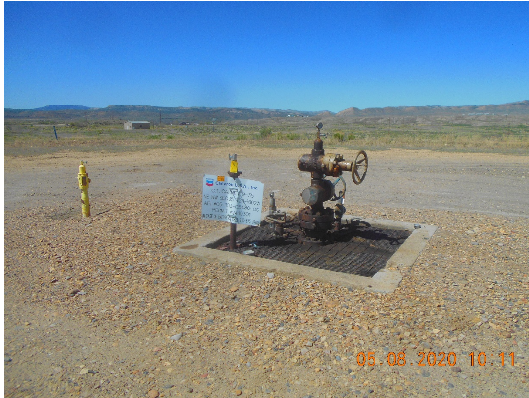
Injection wellhead – Temporarily abandoned
