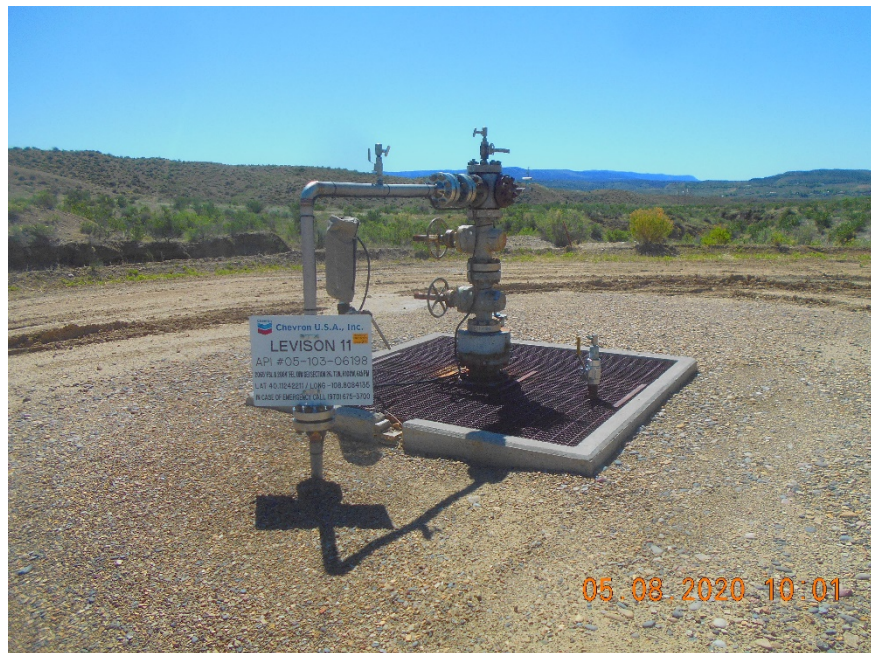
Injection wellhead
