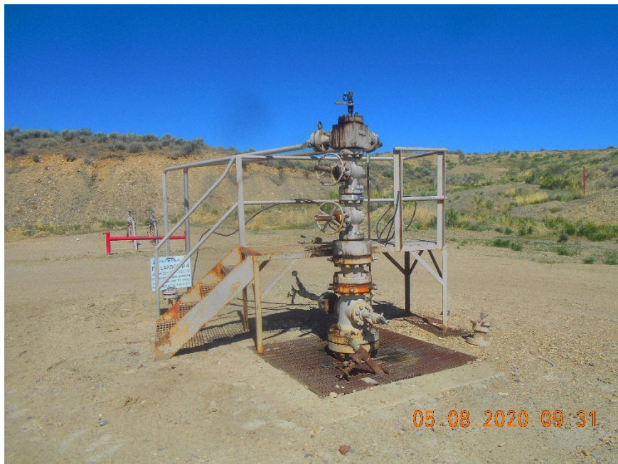
Injection wellhead
