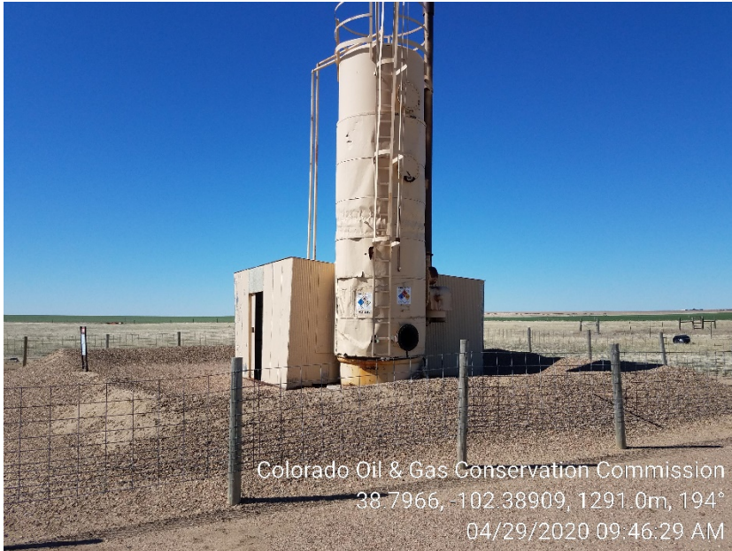
5. Vertical Heater Treater (Not in use)
