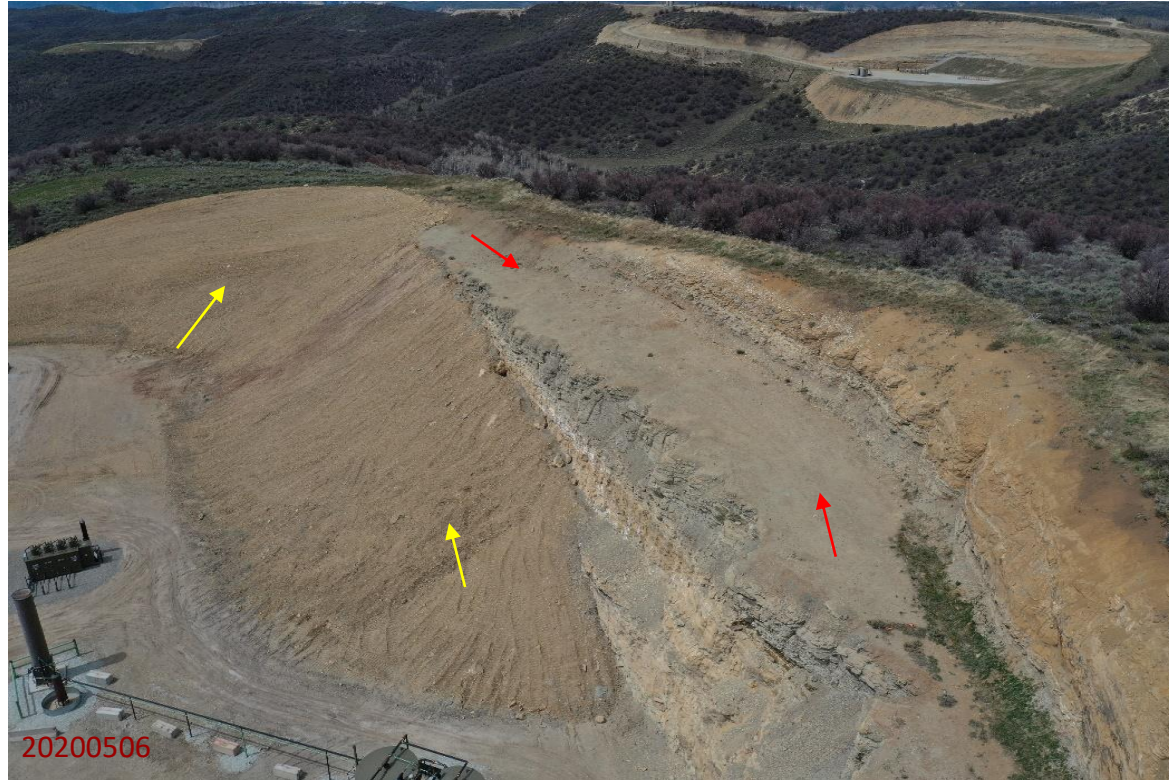
Photo 5: On 5/6/2020, Reclamation specialist Trujillo utilized a SUA to capture aerial imagery of the Location. Photo shows areas on the northern end of the Location where soil replacement/contouring has been conducted (yellow). Photo also shows areas on the northern end of the Location that have not been contoured (red). Photo also shows interim reclamation (revegetation activities) has not been completed.
