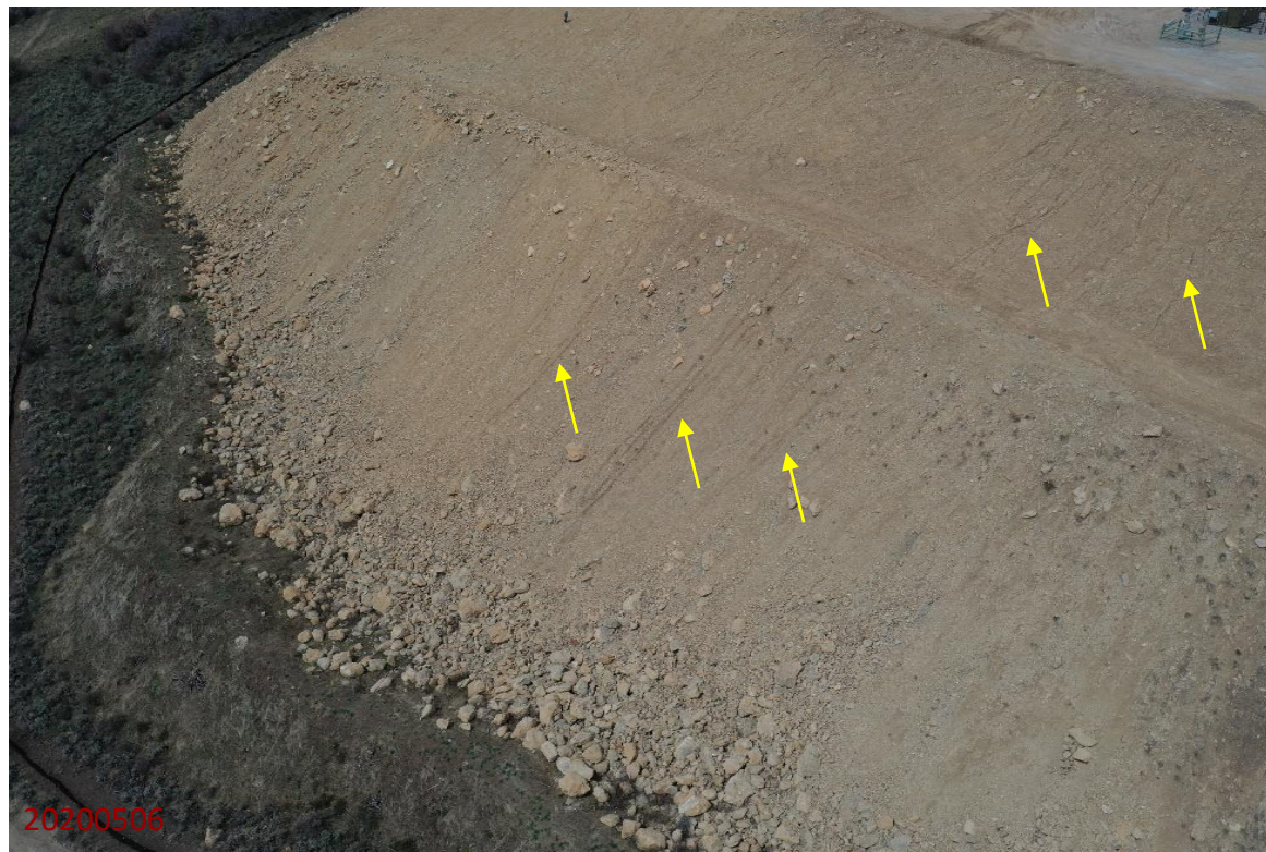
Photo 4: On 5/6/2020, Reclamation specialist Trujillo utilized a SUA to capture aerial imagery of the Location. Photo shows areas where rill erosion/erosion degradation on the southeastern slopes of the Location is evident; BMPs remain missing or insufficient. Photo also shows interim reclamation (revegetation activities) has not been completed.
