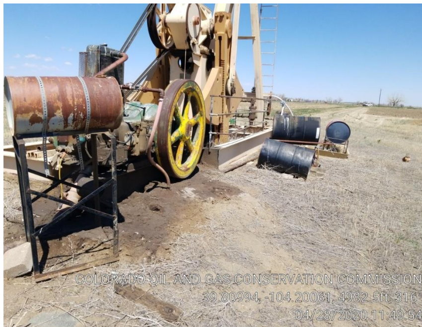
Pic 1 stained soil chemical storage with no containment
