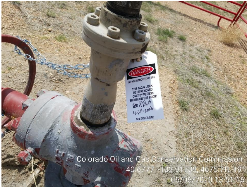
Photo 3 – Well is SI/TA – Install Tags to Comply with Document #401474555
