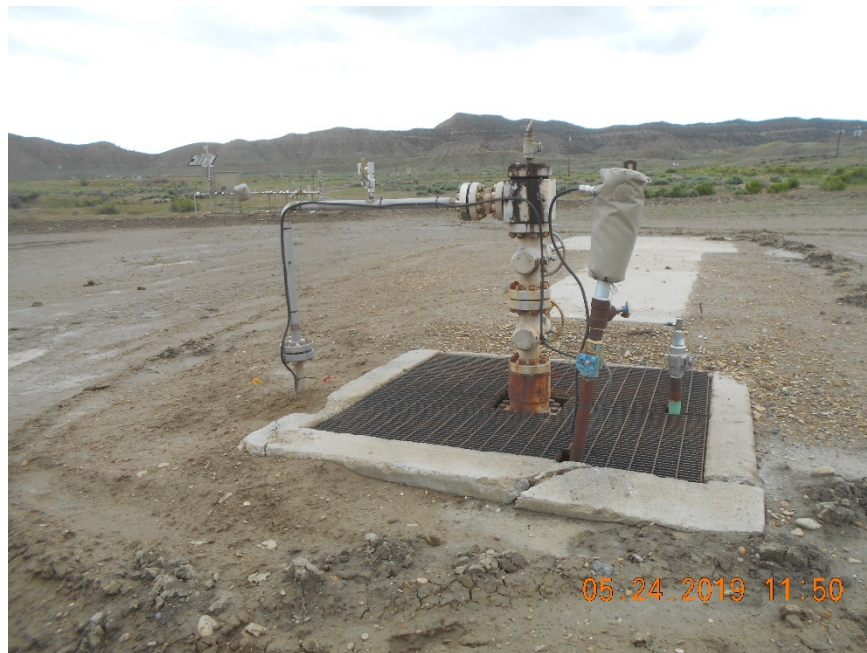
Injection wellhead
