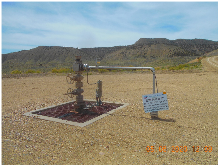
Injection wellhead
