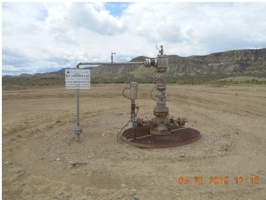
Injection wellhead
