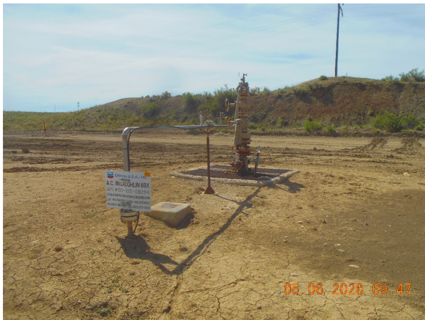
Injection wellhead
