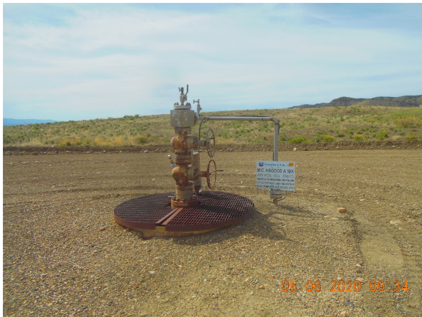
Injection wellhead
