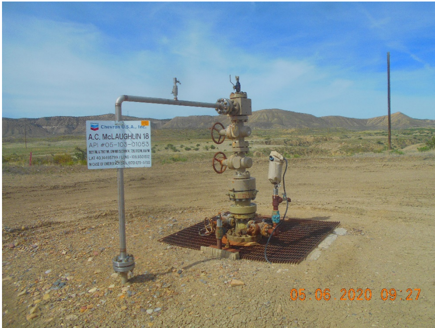
Injection wellhead
