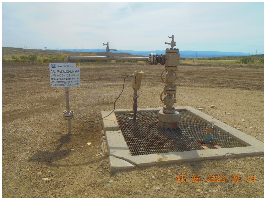
Injection wellhead
