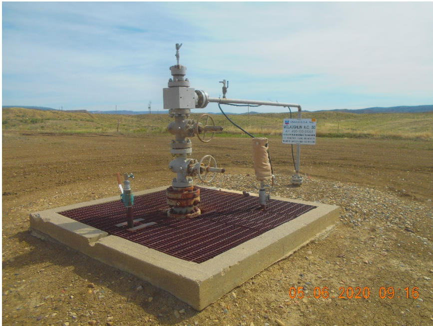
Injection wellhead
