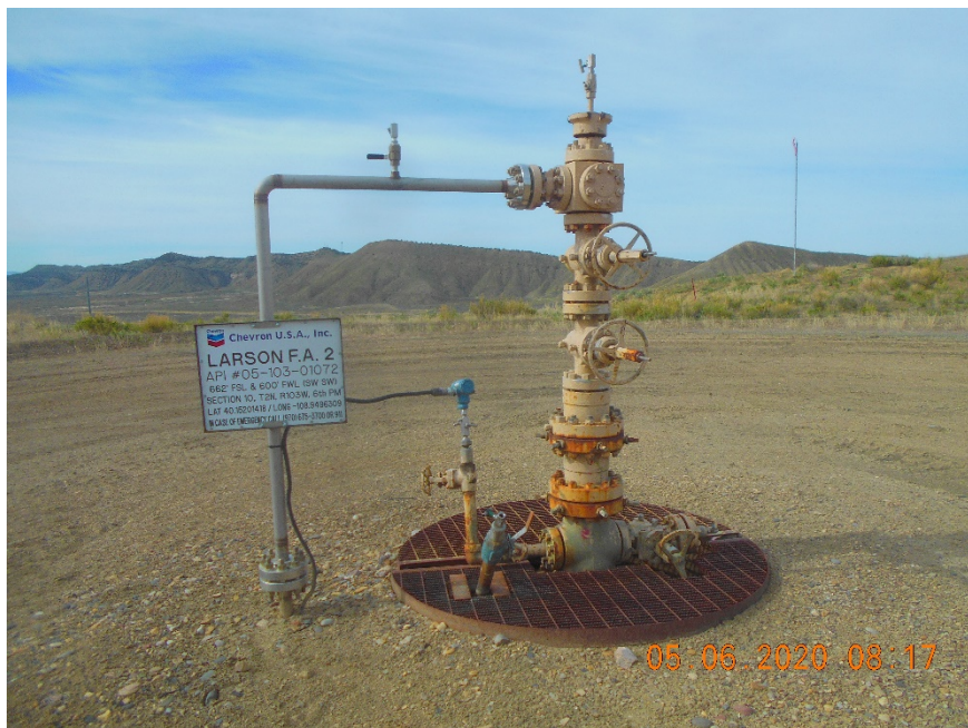
Injection wellhead
