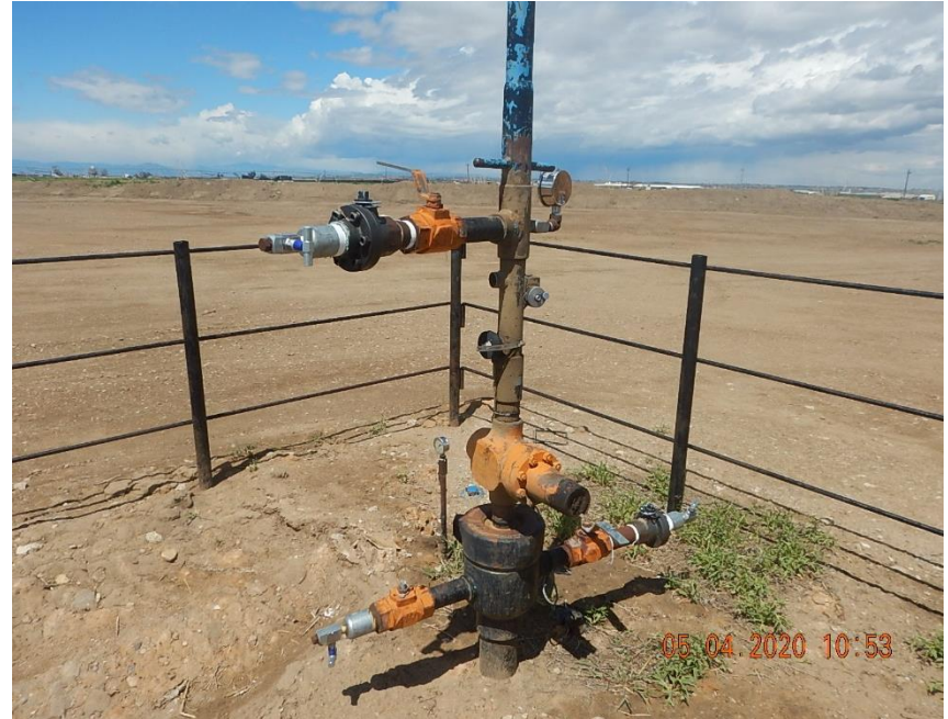
View of (TA) wellhead; Flowline riser removed. Valves closed; bull plugged. View NW
