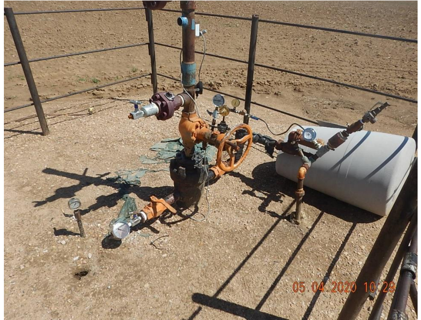
View of (TA) wellhead; Flowline riser removed (hole) Domestic tap/ pressured with casing gas.
