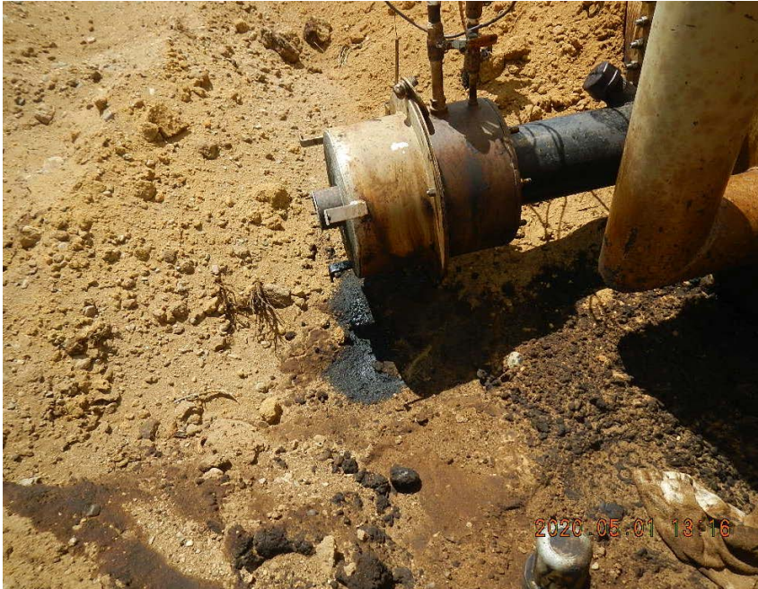
Equipment leaking oil.
