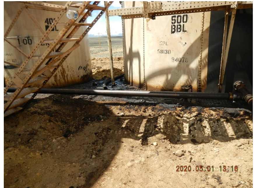
Oil impacts from Spill ID 473059 discovered on 03/09/2020.
