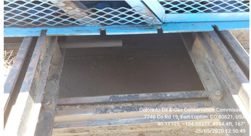
**Photo 7 Stained ground/soil under PU gear box**
