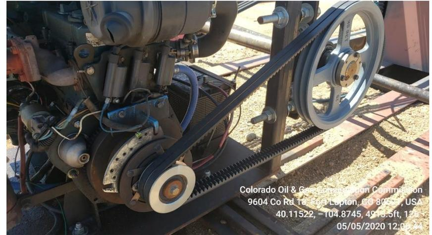
**Photo 5 PU pulley belts have no safety guards covering them**
