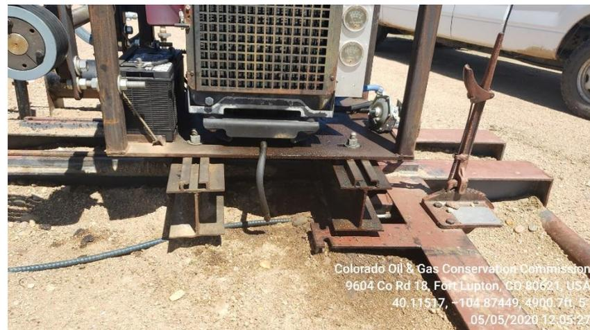
**Photo 4 stained soil under gas engine skid**
